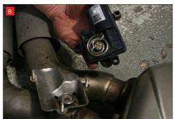
A) After you have removed O.E exhaust you will need to swap the valve motors to the Scorpion exhaust. Remove the 6 nuts
